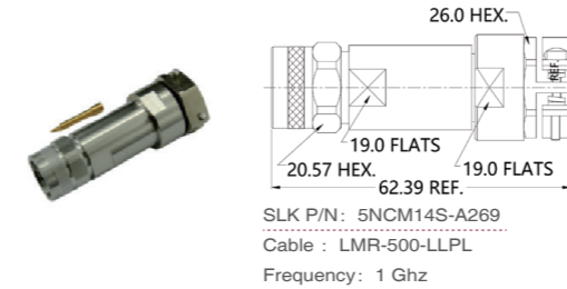
N straight male connector(Flexible cable crimping type)
