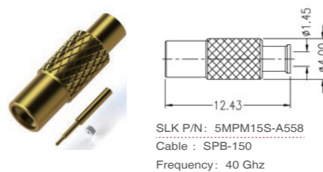
SSMP straight male connector(Semi-flexible cable solder type)
