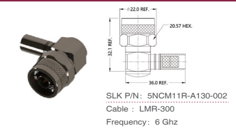
N right angle female connector(Flexible cable crimping type)
