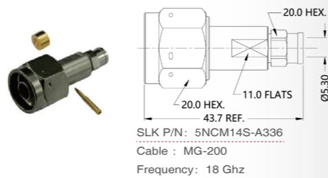
N straight male connector(Flexible cable solder type)
