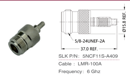
N straight male connector(Flexible cable crimping type)
