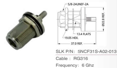
N straight male connector(Flexible cable crimping type)
