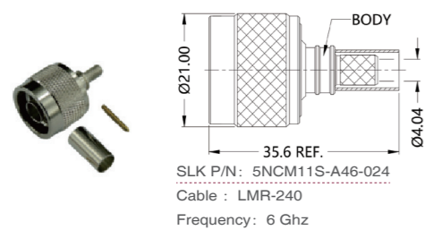
N straight male connector(Flexible cable crimping type)
