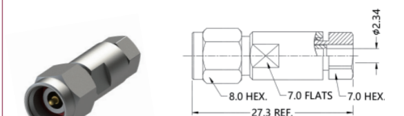
2.92mm straight male connector (Flexible cable solder type)
